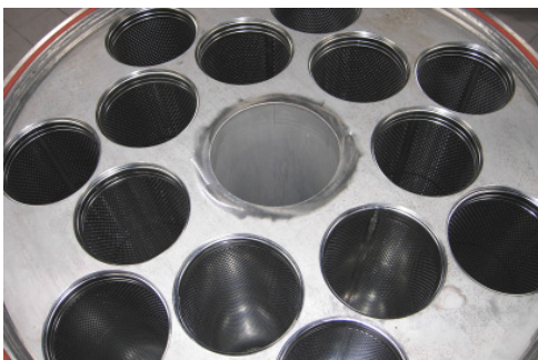
Mounting plate with 14 support baskets for filter bags
